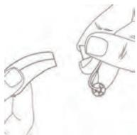
**2.** Pull sound tubing from the instrument by pulling directly opposite from the body of the PAL.
