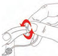
**1.** To remove tubes gently rotate the sound tubing holding the instrument firmly.
